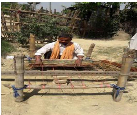
Fig.3: Weaving of mat over a wooden template
