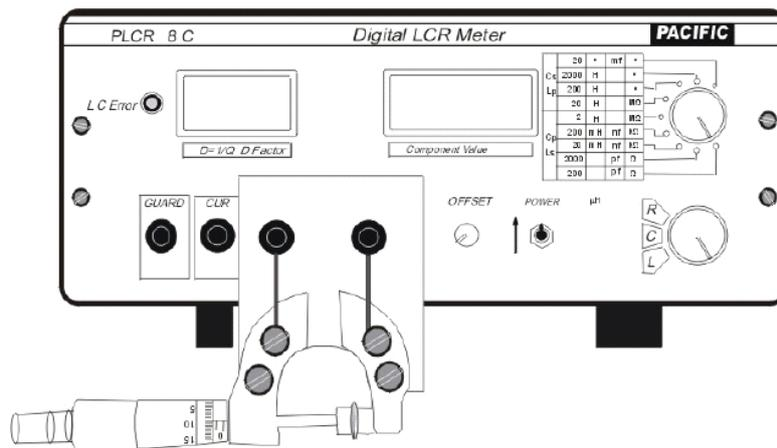
Fig. 6: Experimental set-up for the determination of dielectric properties of Makhana pops.
