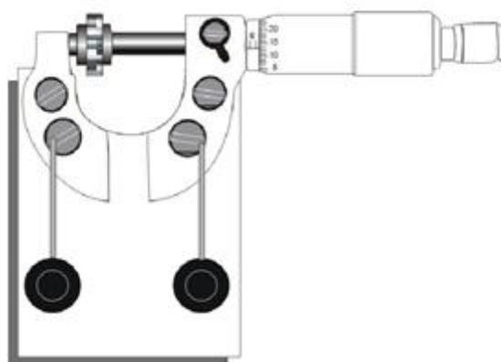
**Fig. 4: Dielectric Cell for the measurement of dielectric properties**
